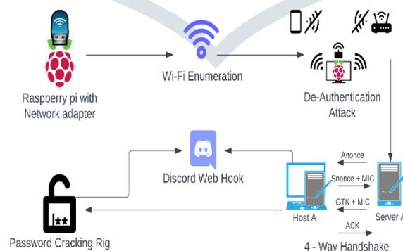
Figure 2: Architecture Diagram
