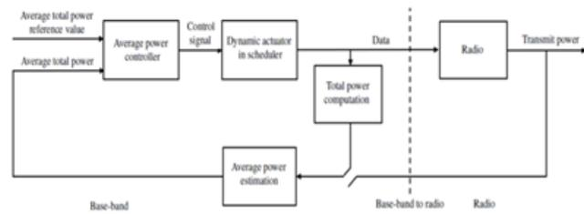
Figure 1: Block Diagram Of The Average Power Feedback Control Loop For The Alternatives With Computed And Measured Momentary Power.
